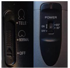
Figure 3.8. Microphone switches to alter the microphone's directionality
