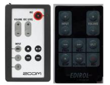
Figure 3.5. Zoom H4n wired and Edirol R-09 wireless remote controls
